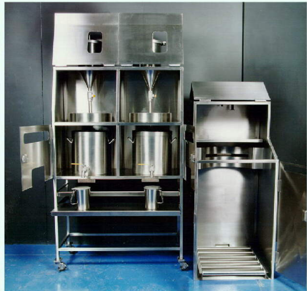
Chloroform and Wax Mixing Cabinet and Drum Enclosure for Tablet Coating
